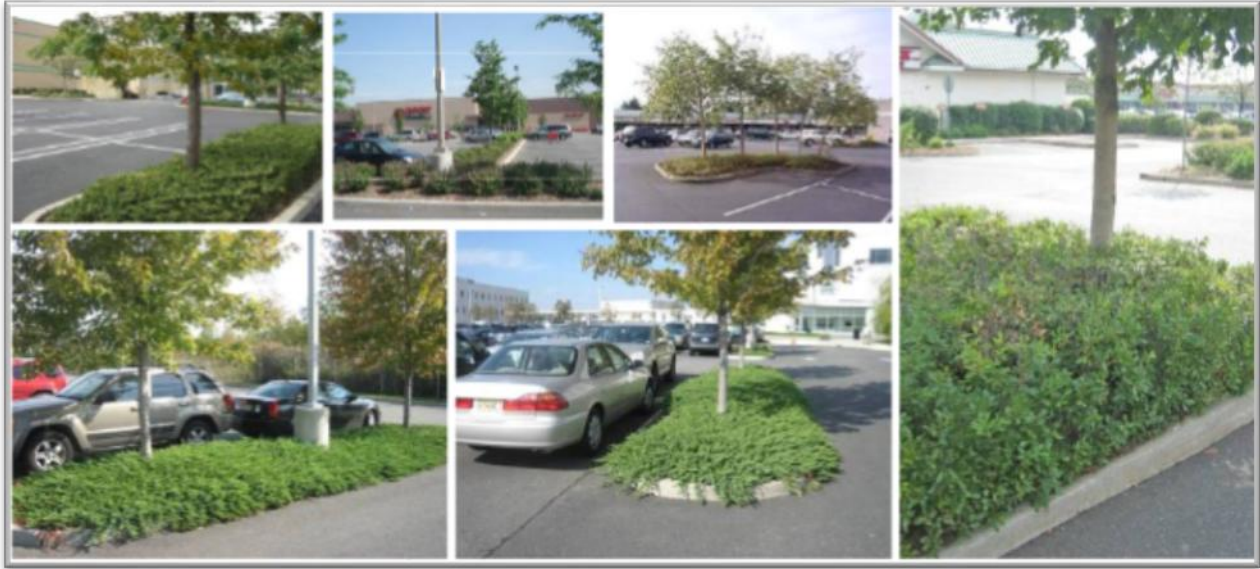
Figure 2: Mitigate expanses of asphalt with plantings that cool the pavement and provide shade and visual interest.
